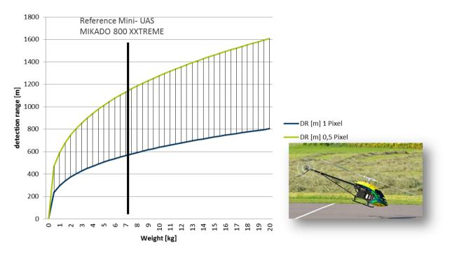
Figure 7: FIRST Sensor detection range, i.e. Mini- UAS
