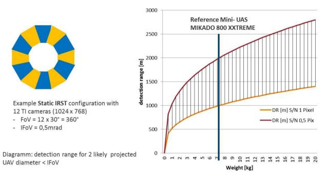
Figure 8: Example Static IRST
