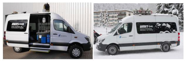
Figure 13: EO- Sensor Suite – mobile test platform MEES & UMIT
