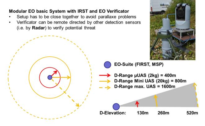
Figure 12: EO-Sensor Suite detection coverage area
