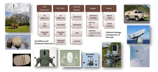
Figure 3: C-UAS Sensor & Effector Options for Engagement Cycle
