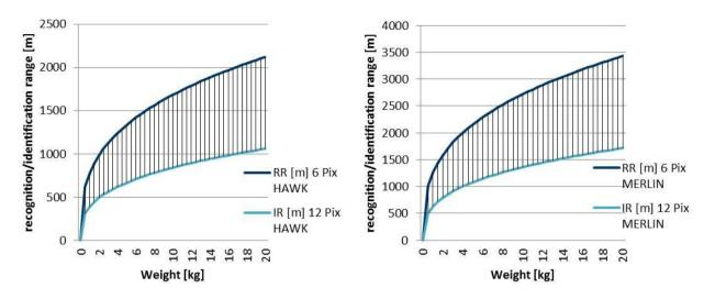
Figure 9: Recognition & Identification Ranges with cooled Thermal Imagers
